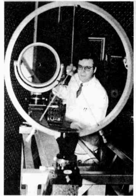
The terminal stations consist of Cassegrainian telescopes having a concave primary mirror behind which there is a laser transmitter or a detector for evaluating the incoming laser light, and a convex secondary mirror (in the foreground). The picture shows the receiving equipment.
