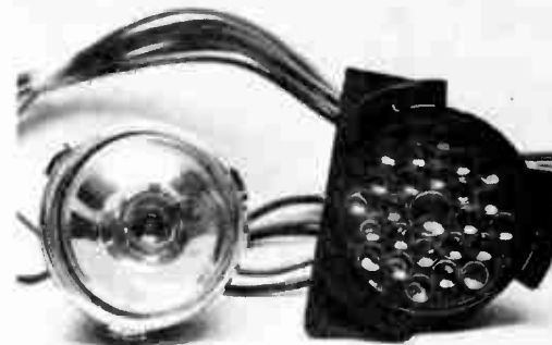
Central light source is divided by 27-way distributor and fibre-optic light guides to provide individual instrument illumination.
