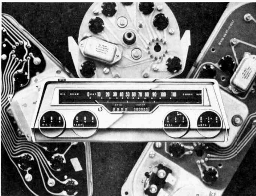
All-in-one instrument panel from Smiths uses printed circuit construction and is connected to vehicle's wiring harness via multi-way plug.
