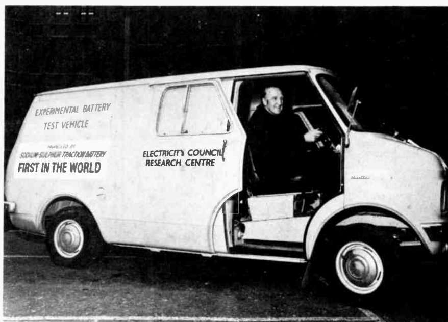
This prototype vehicle built by Britain's Electricity Council's Research Centre is powered by sodium sulphur battery. The battery is one fifth weight of conventional lead acid batteries and gives vehicle a range of 100 miles at 40 mph.
