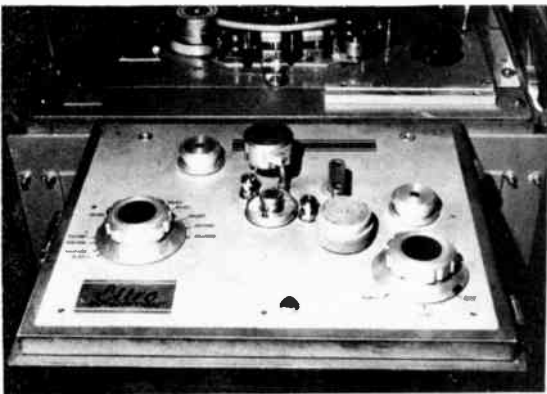
ELTRO 'Tempophon' — Magnetic tape time/frequency compression system.
