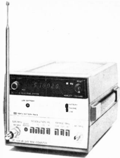
Low current LED digital readout has been chosen by Hewlett Packard engineers for this model 5303B 525 MHz frequency counter.
