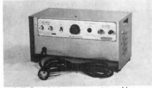
A.C./D.C. variable power supply used by N.S.W. Dept of Education in school science laboratories
