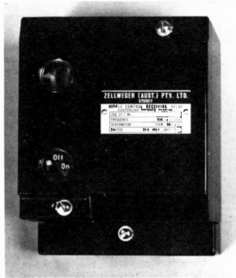
Fig. 9. (a) The Zeltweger ripple control, receiving relay as fitted to the consumer's switch board. (b) The same relay with the main and terminal terminal covers removed.
