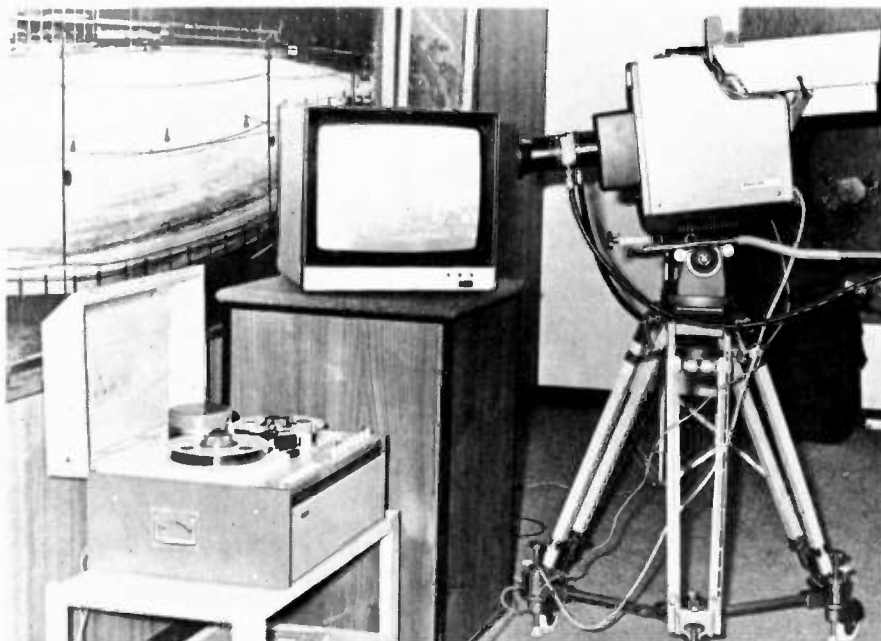
From left to right — the Philips LDL1251 colour video tape recorder, Philips colour monitor and colour camera provide a complete industrial closed circuit system.
