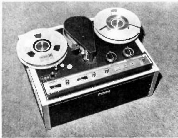
A typical Ampex video tape recorder suitable for production of commercials etc.
