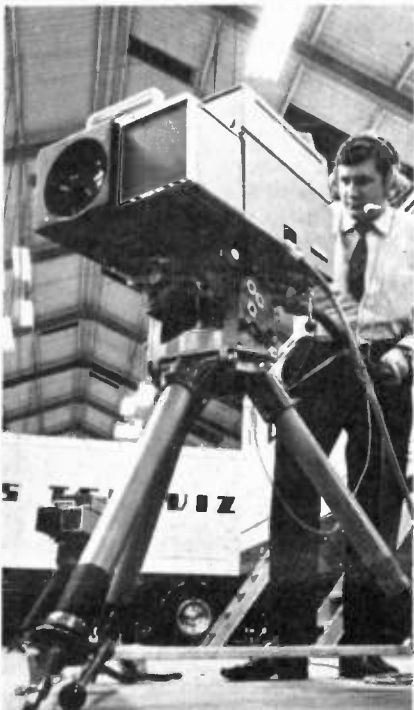
The Marconi Mark VIII automatic colour television camera. A.W.A. Limited are Marconi's Associates in Australia.
