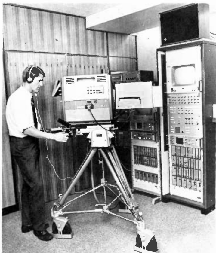
Studio colour camera system from Philips comprises plumbicon colour camera, camera electronics and monitor in rack second from right. First rack provides electronics for "Telecine" 16mm film to television system.
