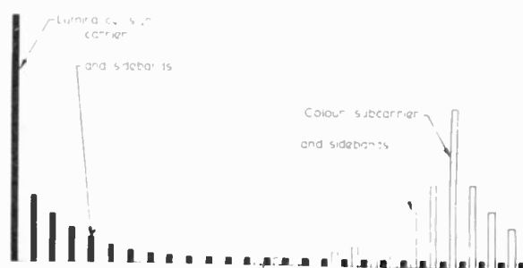
Fig. 2. Diagram showing how luminance and chrominance signals are interleaved to give a bandwidth equal to that of black-and-white television.
