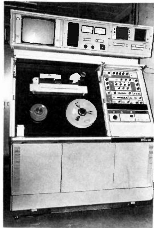
The Ampex AVR-1 studio video tape recorder uses 2" tape and automatically locks up to tapes produced on NTSC, PAL or SECAM systems.
