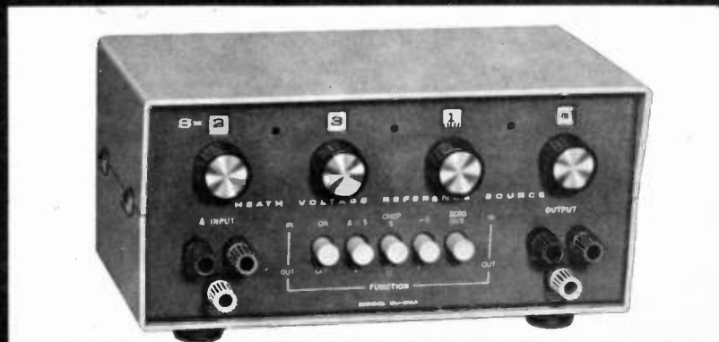
HEATH EU-80A AC/DC CALIBRATOR
