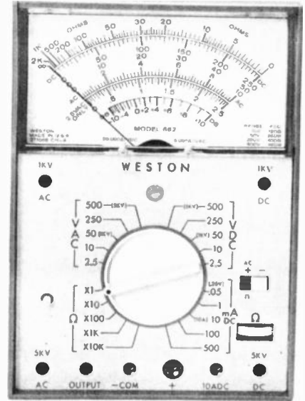
Another in the Weston 660 range, this 662 VOM features passive circuitry. It has the same "droppable" characteristic of all the 660 range of instruments.
