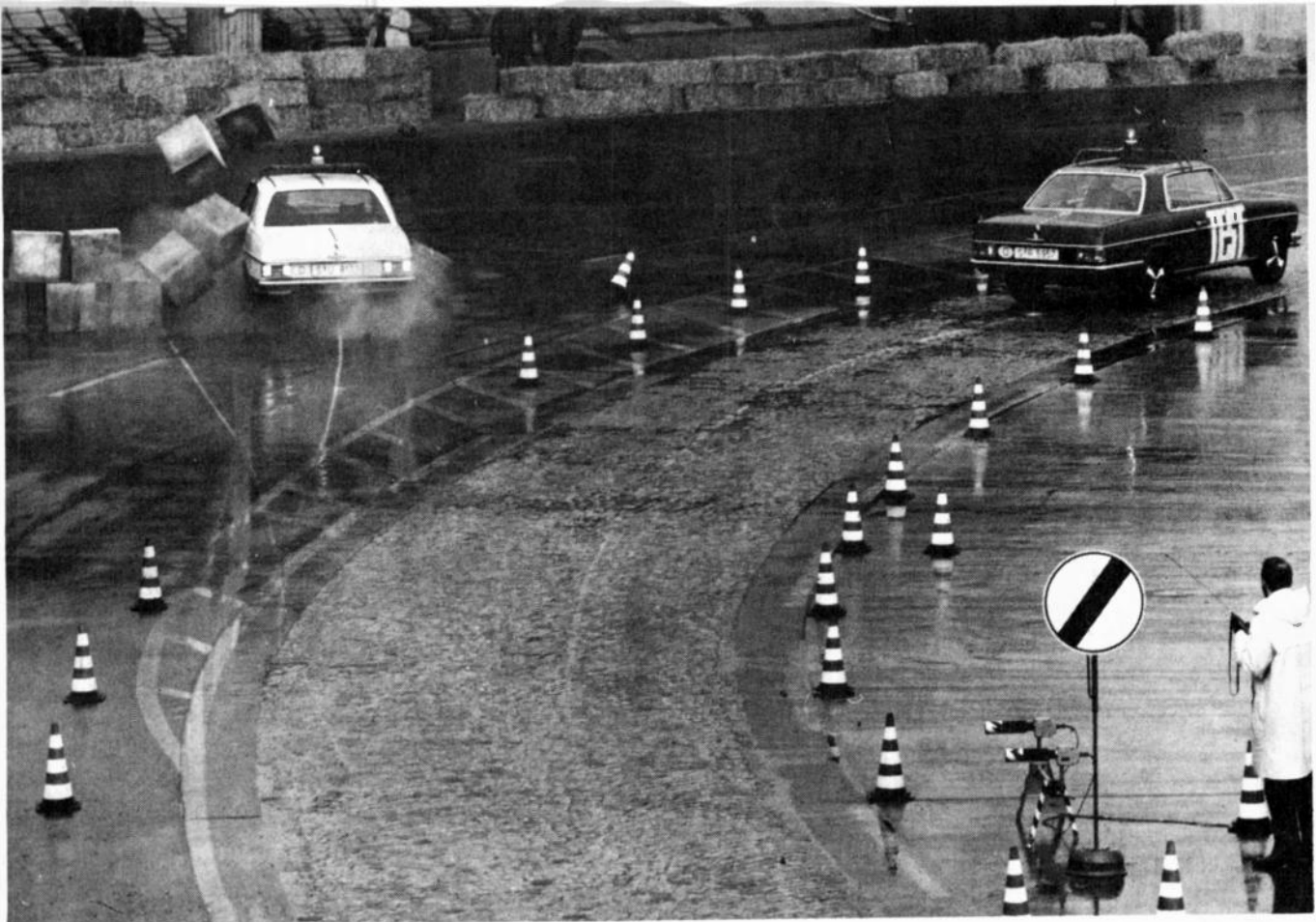
The black vehicle has electronically controlled braking.
