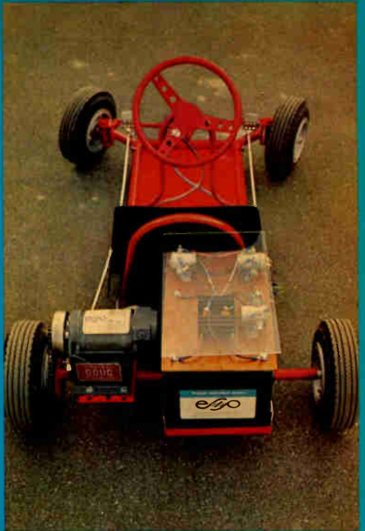
ABOVE: Originally the first, this is now one of 35 stations with charging facilities for electric cars between New York and Los Angeles. RIGHT: Lead-cobalt battery powers this 40 mph, 150-mile range EFP chassis. BELOW: Converted Renault recharges in 45 minutes, has 70 mph top speed.
