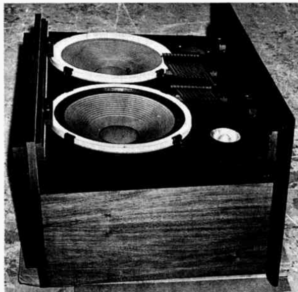
Speaker with grille removed. Woofer is at rear of photo, passive radiator at front, high-frequency components at right.
