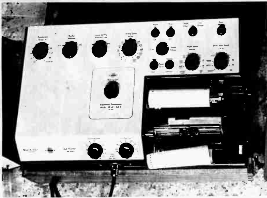
Bruel & Kjaer level recorder provides graphical record of output at varying frequencies. Sample graph below was taken during our test of Sansui Quadphonic Synthesiser (see report, page 64).
