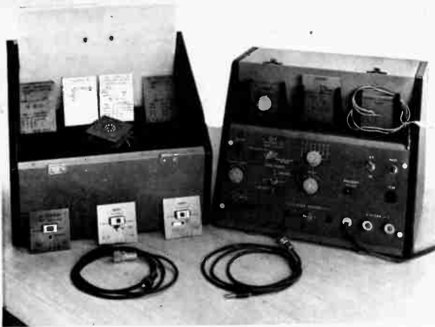
Characteristic curves of a wide range of semiconductors can be displayed with the aid of this CIT curve tracer.
