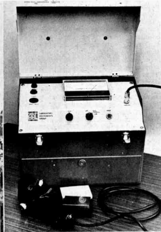
ARL hardness tester utilises piezo-electric transducer. Left, complete unit; right, schematic drawing and a cutaway of indenter head.
