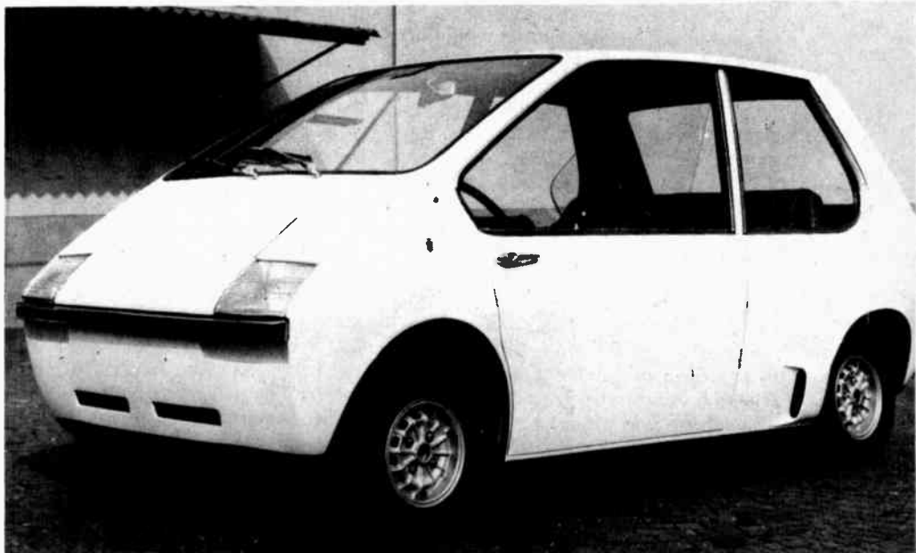
Rowan city car shown at Electric Vehicle Symposium in Phoenix, Arizona, had 60 mile range. Fuel costs were less than one-third of a cent per mile.
