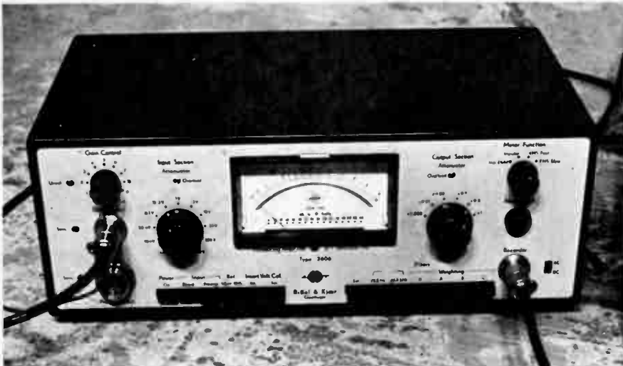
Measuring amplifier takes flat or weighted measurements of energy from 2Hz to 200kHz.
