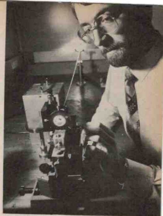
Dr Ken White of the British Post Office Research Station making optical measurements on a length of optic fibre. (Picture courtesy of the BPO).
