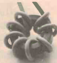
To prevent RF pickup in signal-carrying cables, wrap them around the core of a small ferrite toroid.
