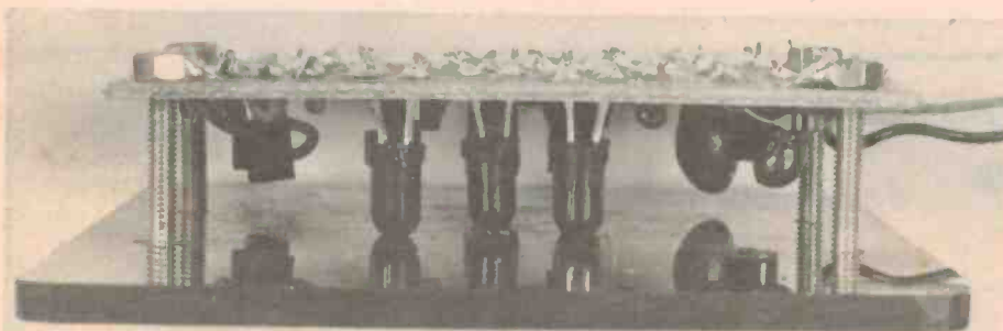
This picture shows how the pc board is mounted behind the red perspex front panel. The LEDs should sit close to the perspex.
