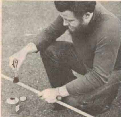
Cut the spreaders to length and weatherproof with Linseed oil or other sealer.
