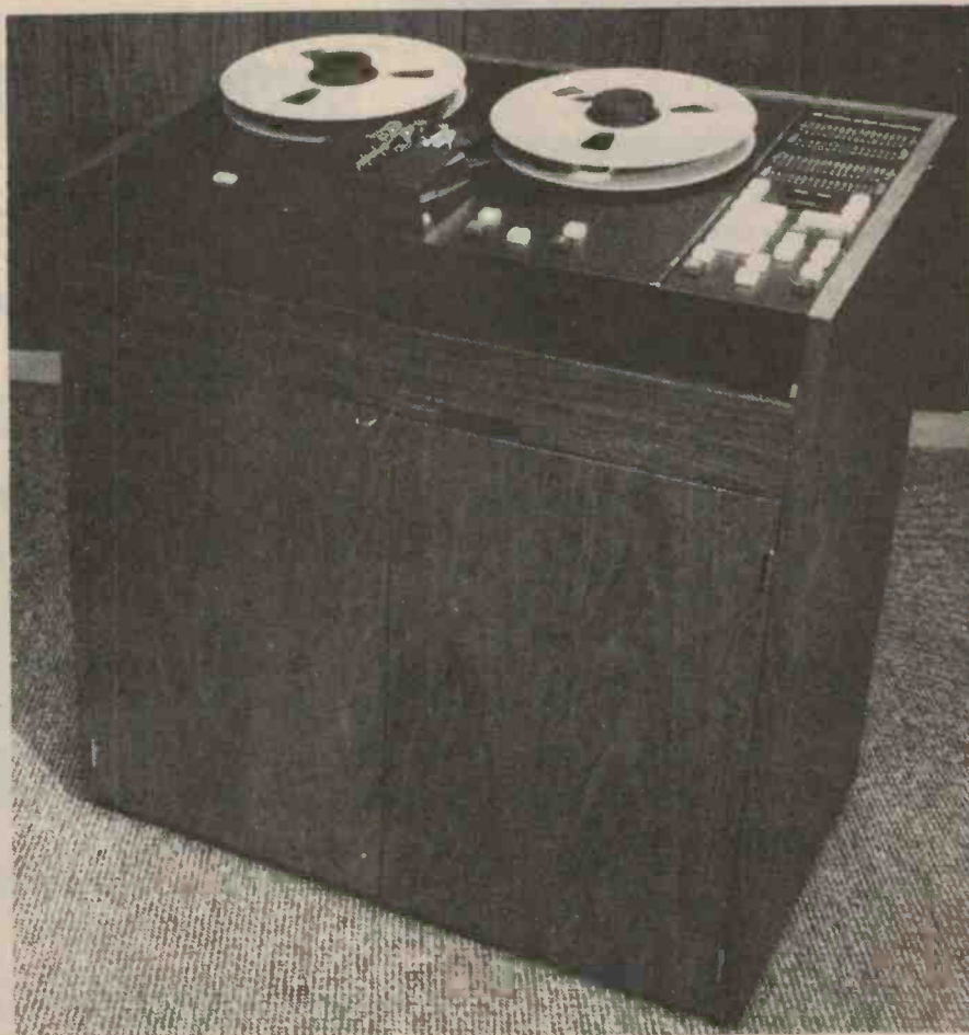
The most sophisticated of the professional digital recording systems is this piece of equipment from 3M. Designed for studio use, it was developed jointly with the BBC and can record 32 tracks of 16-bit information on a 25 mm tape running at 1143 mm per second. Sampling of the input is at a rate of 50 kHz (i.e. 50 000 samples per second). Frequency response is within 0.3 dB between 30 Hz and 15 kHz, signal to noise ratio is claimed to be not less than 90 dB while distortion is said to be better than 0.03%.
