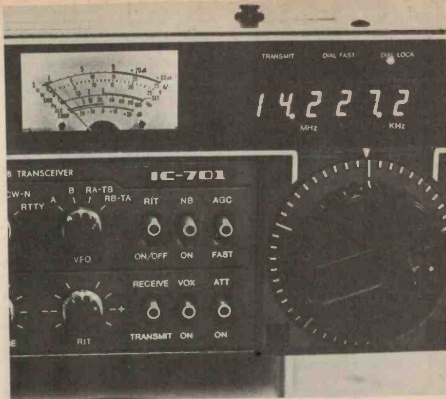
The distinctive dial, centre position S-meter and control groupings make the Icom IC-701 stand out amongst the many transceivers on the market. The split transmit-receive frequency facility, provided by the 'VFO' switch is a feature that comes in very handy when trying to work DX through a dog pile. The RIT control — equivalent to the usual clarifier — can be selected to operate on both the transmit frequency and the receive frequency.
