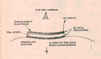
Direct viewing of the state of the 'aura' of a living object using a transparent electrode.
