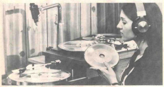
Kitty Puckett checks out 45 rpm stamper, while auditioning one at 331/3 rpm.
