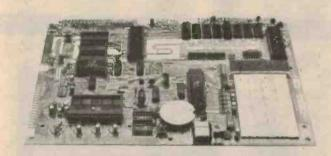
A sure starter in performance. In quality. In availability. OEMs, educators, engineers, hobbyists, students, industrial users: Our Versatile Interface Module, SYM-1, is a fully assembled, true tested and warranted microcomputer board that's a single-board computer, complete with keyboard and display. All you do is provide a +5V power supply and SYM-1 gives you the rest.
