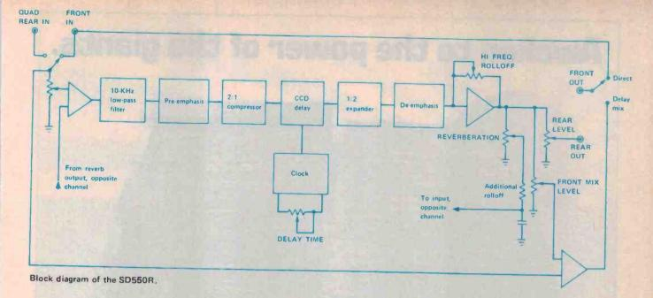
so for realism in the listening room the delayed signal should also be attenuated at the top end. The SD550R uses a bucket-brigade device to generate its time delay - and bucket-brigade systems have a natural roll-off at high frequencies. A high frequency roll-off adjust is provided and is calibrated from -3 to
