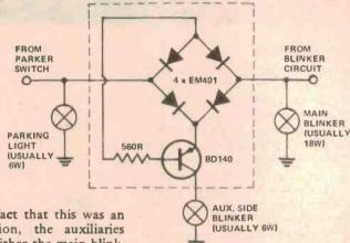
Kris spotted the fact that this was an exclusive-or function, the auxiliaries coming on when either the main blinkers or the parking light was lit, but not if both were lit. He devised the circuit here which he then fitted into a plastic pill bottle (useful things) and inserted into the wiring at each side of his car.
