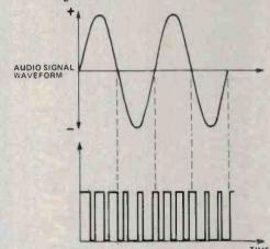
Fig. 3. Class D amplification uses pulse-width modulation. Pulse amplifiers are very efficient and the pulse-width modulation process can be made very linear.
