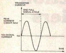
Fig 1. In a Class, A amplifier the transistor is on and conducting for the duration of the signal waveform. The no-signal current is quite high and the class A amplifier draws power all the time.
