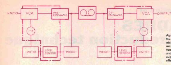
Figure 1. Basic block diagram of the ADRES noise reduction technique. During recording, the incoming signal is compressed as a function of the frequency range and input level. On playback, expansion counteracts this, effecting a reduction in noise.
