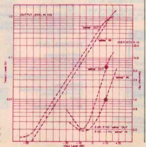
Figure 4. Toshiba claim a considerable reduction in third harmonic distortion when ADRES is used.
