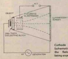
Cathode ray tube arrangement (schematic only) for picturing the field around the object being examined.
