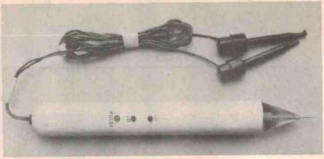
The completed logic probe.
