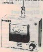
The field strength meter enables day-to-day checks of radiated power, comparison of different antennas and the plotting of radiation patterns.
