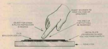
Figure 6. Simple method for making Kirlian photographs of fingertips using static charge built up on the body.
