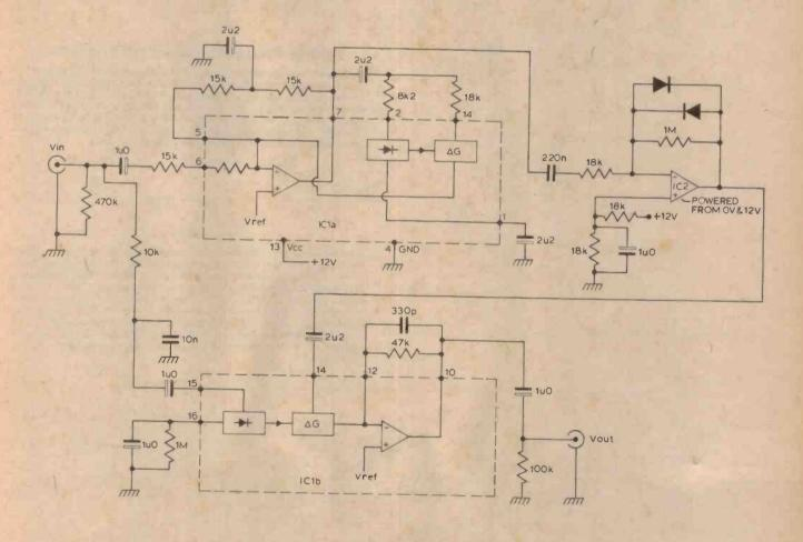
Fuzz boxes are used by guitarists to produce harmonic distortion and sustain. If you want to produce only the distortion, but to retain the original envelope of the signal then this is the circuit for you.
