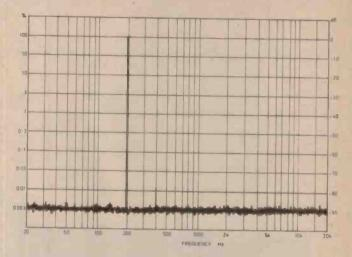
Fig. 3 Spectrogram of the 200 Hz drive signal, suppressor switched out.
