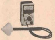
The HI 1501 is a rugged, compact, portable instrument and is virtually immune to failure caused by excessive fields or physical abuse. It consists of a lightweight instrument package connected to a unique detection probe by a shielded cable.
