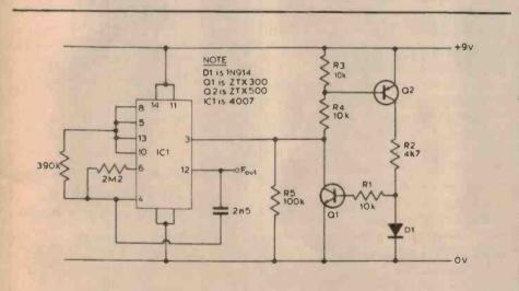
Temperature to Frequency Converter This circuit uses the fact that when fed from a constant current source, the forward voltage of a silicon diode varies with temperature, in a reasonable linear way.
