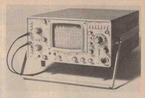
The BWD 540 (above) is an Australian-made high performance dual trace oscilloscope.
