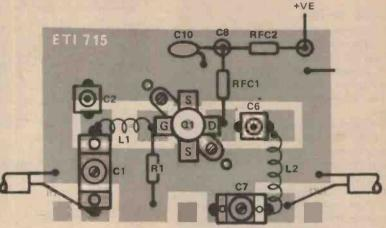
Fig. 2. Component Overlay.
