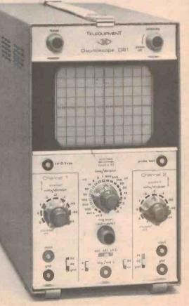
plete trace each time. In the third method the beam draws both traces in one sweep by alternating very quickly between traces. In this "chopped" mode the beam may draw say .1 mm of the top trace, then .1 mm of the bottom one, then back to the top, etc.
