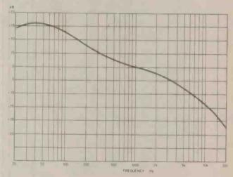
circuit overall demonstrates an input overload threshold of about 37 dB at 1 kHz ref. 2 mV input.
