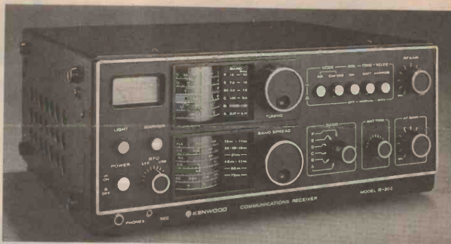
A good example of the use of a separate bandspread dial is the Trio Kenwood R300.
