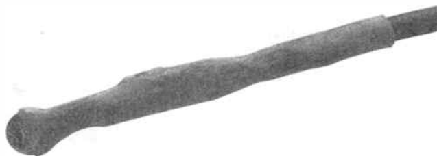
View of the thermistor assembly, used to sense the battery temperature. The connections are sleeved in heatshrink tubing, then the whole assembly sleeved with more heatshrink tubing for protection and rigidity.
