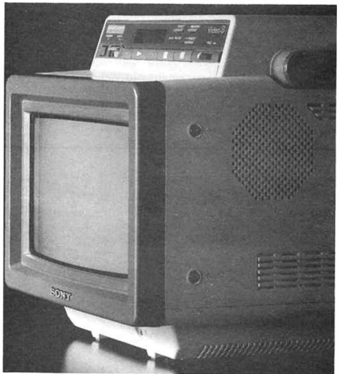
Sony seems to be the only supplier of a 12 Vdc operated colour video monitor. This is their EVM-9010, a 9" (230 mm) screen unit with integral 8 mm video cassette playback unit. Sony's HandyCam video camcorder with a "Sports Pack" or "Marine Pack" is ideal for the boating enthusiast keen on recording boating activities.
