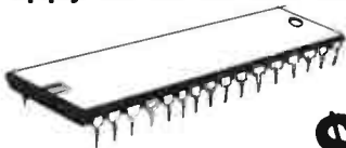
Western Digital 2793A. Single rail, single chip, floppy disc controller.
