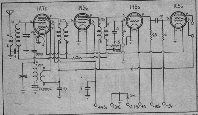
The circuit uses as few parts as possible. No alteration from standard practice is needed for the new valves. The 1H5G has its grid returned to earth.
