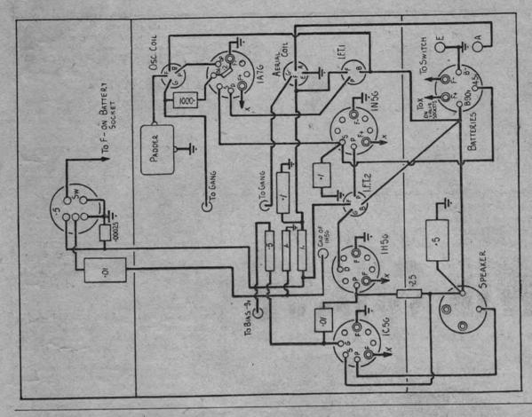
This wiring diagram shows details of layout and connections. It is drawn to scale, so you can make measurements from it.
