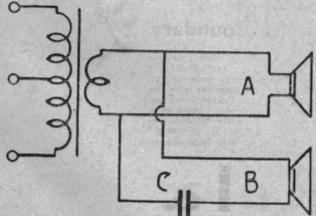
Fig. 1.—How the speakers are connected together with the voice coils in parallel. Speaker "B" is a permagnetic type.
