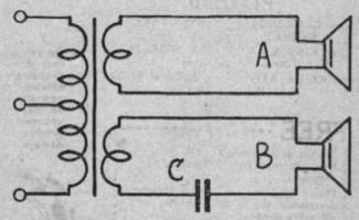
Fig. 2.—How a transformer may be used with two secondaries, should the speakers have different voice coil impedance.
