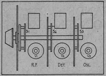
Illustrating a suitable layout where switching is applied to a set having an R.F. stage.
