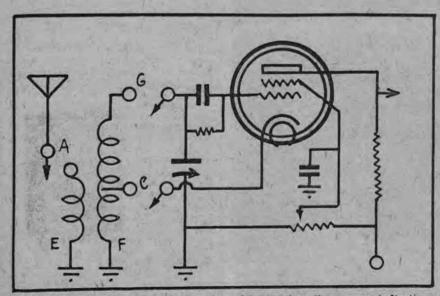
A skeleton circuit of a detector valve with reaction, the arrows indicating where the switching takes place.
