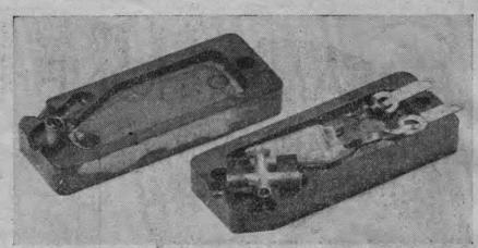
A photograph of the crystal cartridge opened up. Note the needle chuck jastened to the crystal.
