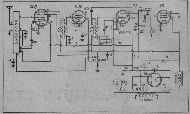
Schematic of the circuit. It will be noticed that the circuit is a modified "Advance 1937."
