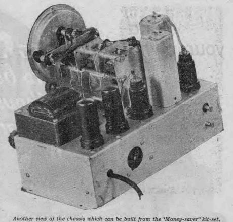
In the rear of the base can be seen the valve socket into which the speaker plug connects. The set should not be switched on unless the speaker has been plugged in. Wireless Weekly, March 18, 1938
