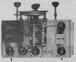
Plan view of the chassis, showing the values fitted in their respective sockets. This photograph also gives a good idea of the three wires which are above the base.
