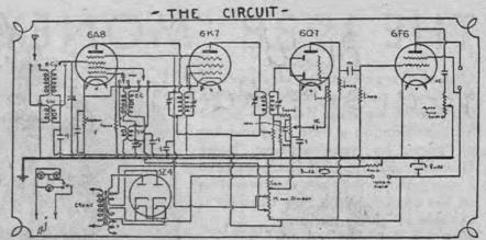
Circuit diagram for the "Money-saver." It should be noted that in addition to the valves shown in this diagram it is also possible to use the octal-based glass equivalents, type 6A8G, 6U7G, 6B6G, 6F6G, and 5Y3G.
