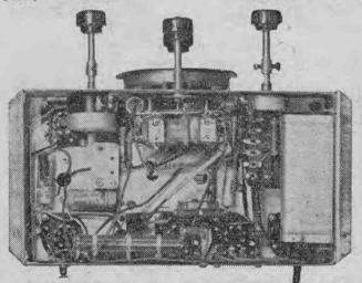
A view showing the wiring of the chassis. This photograph can be used in conjunction with the picture diagrams to show the components and their correct positions in the assembly.
