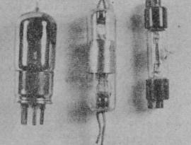
Left to right: The so-called "Dutch" valves used about 1924. Next is the "Audiotron," the first valve available here to ama-teurs, about 1920. The third is the "Myers" valve, used in receivers about 1922. The "Audiotron" had two filaments in case one of them burnt out!
