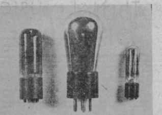
Left to right: The UV199, the first American "dull-emitter" valve. Next to it is the 201A, a famous valve about 1926. The little chap is the "Weco-valve," one of the early dullemitters of midget size.
