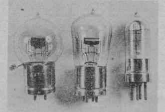
A collection of popular "bright emitters" about 1924-1926. First is the D6 double grid valve, the forerunner of the pentode. Next is a standard triode, the D4. The valve with the hood-shaped plate is the jamous P1. All these are 4-volt valves
