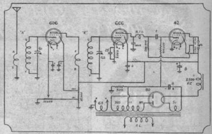
Modified circuit to obtain greater selectivity by omitting the grid leak and condenser and fitting a cathode bias resistor and by-pass to the detector.
