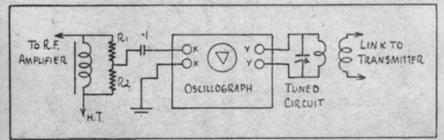
Showing how the oscillograph is connected for a trapezoidal pattern. R1 is 2 megs, and R2 is 100,000 ohms in our case. Sometimes a stabilising resistor of 10,000 ohms is wired between the terminals marked YY. A check on the modulator wave form may be made by leaving the connections undisturbed and switching over to the 50 cycle sweep.
