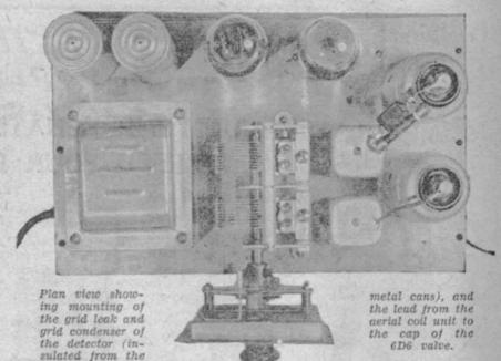
it were the centre terminal of the other style of condenser, and it is the black lead which will be connected to the metal of the base in one case and insulated from it in the other, running to the 300 ohm bias resistor.
