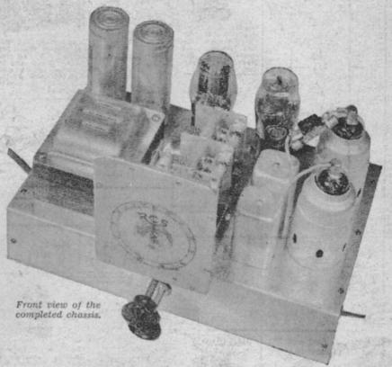
The receiver is for the broadcast band only, and is not a dual-wave model. It is not fitted with automatic volume control or any of the modern gadgets. It is just a straight-out receiver, designed to be simple to build, to be cheap in cost and to offer value for money. The original has been carefully tested in our laboratory and we have spent considerable time testing out alternative detector circuits, and all manner of modifica-
