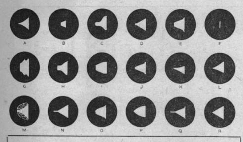
A—Plate modulated with excessive bias or regeneration.
