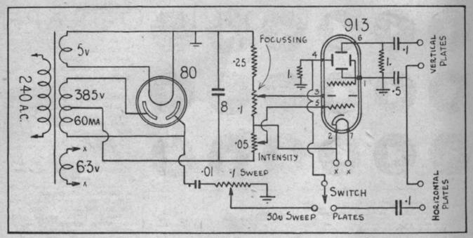
The circuit. The numbers on the 913 indicate socket connections. No. 8 pin is connected internally to No. 1 pin, and is therefore left blank.
