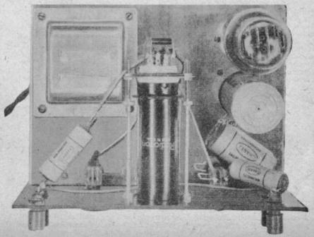
A photograph of the oscillograph from above the chassis. Note the & watt 1 meg. resistors wired right at the socket,
