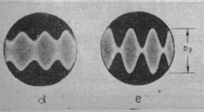
Modulated envelope patterns showing (d) partial modulation, and (e) 100 per cent. modulation.
