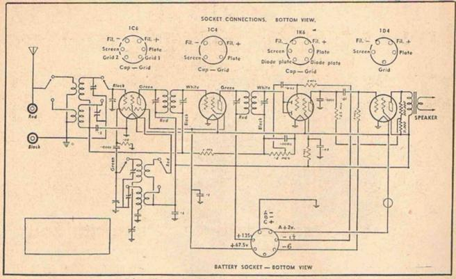
Schematic circuit, with socket connections shown above. ment of the switch will call for a cer-
