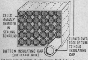
Cut-away view of bottom of solid Battery Block before insertion into Battery Box. Note how the bottom of each cell is completely insulated and protected.
