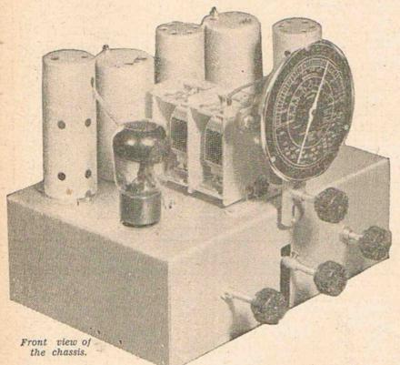
In this article we describe what may be considered the standard four-valve receiver for 1937. It has all the features of its predecessors, in addition to several modern improvements, including universe feedback. It is an ideal receiver for use with the new Air-cell.
