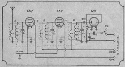
The circuit schematic diagram, showing the pick-up switch.
