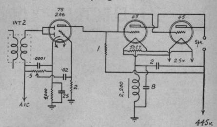
Portion of the circuit used by a prominent manufacturer for the 1937 models, showing the use of a 75 or 2A6 type valve as diode detector, and a.v.c. valve with direct coupling to the grids of the output valves.
