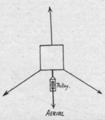
Diagram showing direction of pull of the aerial and the middle and top sets of guys. The lower set of guys consists of only a pair arranged at right angles to the thickness of the lower section of the mast.
