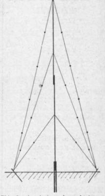
This drawing is to scale, and gives a good impression of the slender appearance. The stakes for the guys should be at least ten feet out from the foot of the mast.
