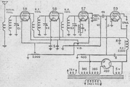
Here is a circuit of a T.R.F. set, actually termed the Standard Midget, and published some time ago. We give the circuit in response to several requests of late. The coils used are standard T.R.F. coils, and matched for the particular tuning condenser used. The set will be found easily equal to separating local stations, and also has excellent sensitivity where needed. It is also very inexpensive to make.
