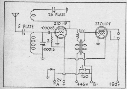
The Paris Two is still one of the most popular of small two valve short-wavers. Here is the original circuit, with all values marked. The coils should be wound on 11 inch formers. To tune from 15-35 metres, use 5 turns for the grid and 8 turns reaction. For 35-55 metres, use 10 turns grid and 12 turns reaction. For 55-90 metres, use 20 turns grid and 15 turns reaction. Almost any wire would serve, a good suitable gauge being 22 d.c.c.
