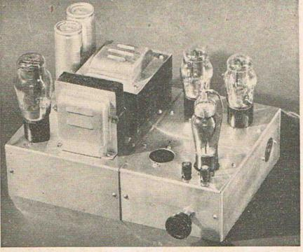
The amplifier and power supply unit. The vacant socket will be used for a microphone pre-amplifier valve.
