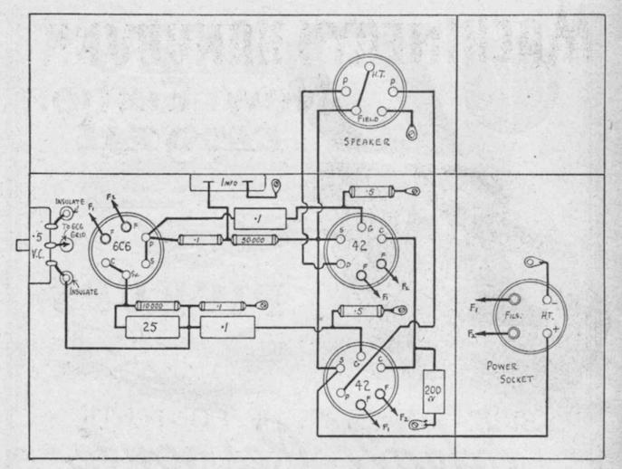
Wiring diagram of amplifier.
