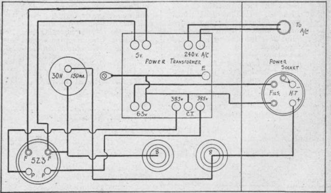
Wiring diagram of power supply unit.
