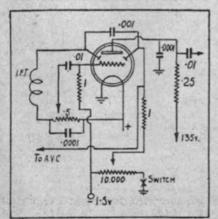
How a sensitivity control may be fitted for fine adjustment.
