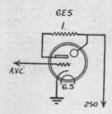
a fluorescent material. Electrons impinging on the coated target cause it to glow. The extent of the fluorescent area can be controlled by means of a third electrode placed between cathode and target. The pattern developed on the fluorescent target depends on the contour of the target as well as on the position and shape of the third electrode.
