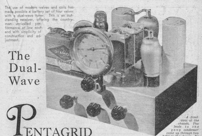
HE development during the last few months of more and more efficient coil kits, and the introduction of better valves, has at last made possible a four-valve battery dual-wave receiver, which we consider thoroughly satisfactory.
