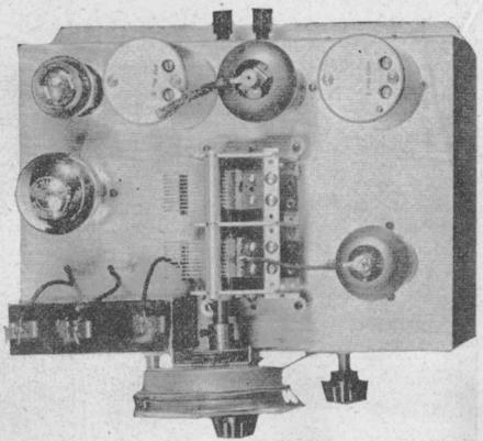
Looking down on the chassis. Note "C" battery connections, and shielding of I.F. valve plate lead.
