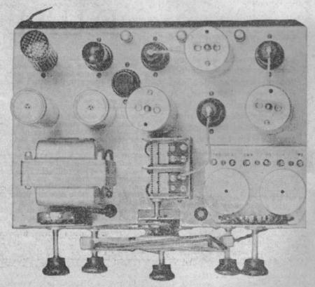
This view of the layout of the base also shows the mounting of the dual-wave unit, with its row of trimmers and padders mounted at the rear.
