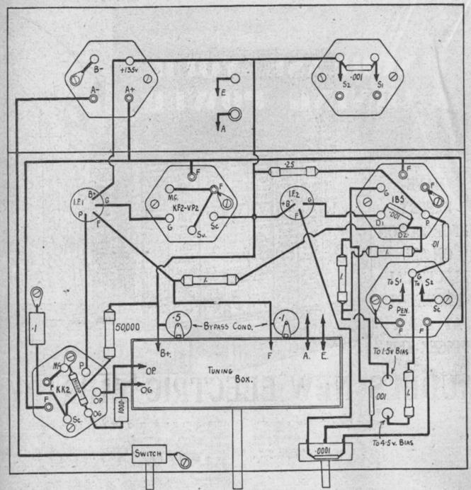
All wiring under the chassis is shown here. Note the two bypass condensers, which are placed vertically right at the tuning box.
