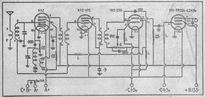
All components are marked in this circuit diagram. A fixed condenser of .0001 from the 1B5 plate to chassis is an optional component.
