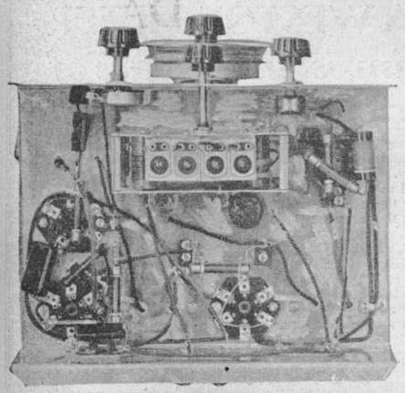
A view of the components under the chassis of the actual receiver.
