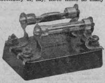
A Resistance Coupler—the condenser is in the base. Separate components are often used.
