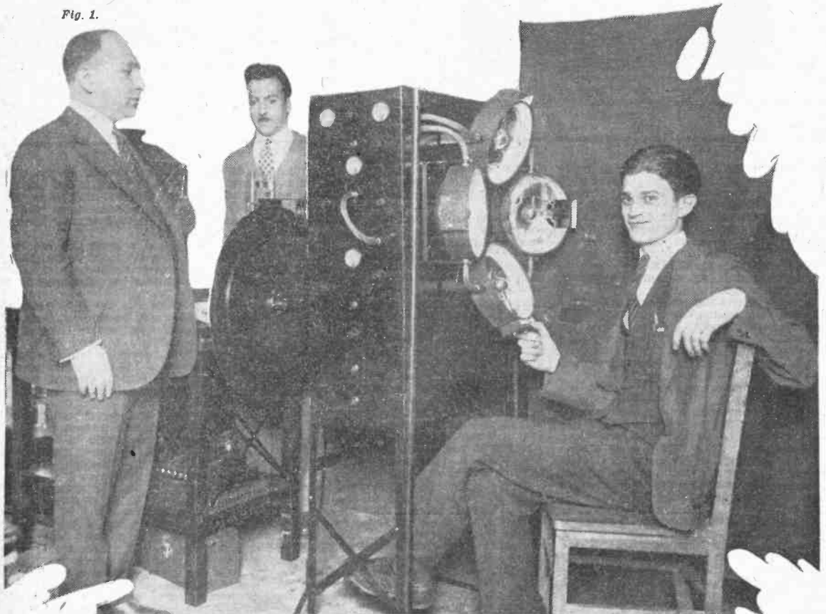
The television transmitter erected by the Pilot Company. Mr. Geloso, the author of the article, is seen seated before the televisior.
