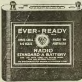
"STANDARD" "A" BATTERY. Price . . . . . 9/. The Ever-Ready "Standard" "A" Battery (3 cell) 4.5 volt, specially designed for economical operation of 1, 2 or 3 valves, taking .05 amperes at 3 volt. For sets with four or more valves, the most economical service is obtained by using two "Standard" "A" Batteries connected in parallel.
