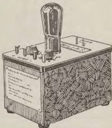
High tension supply unit
