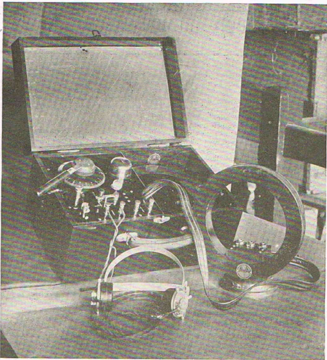
Wavemeter designed and constructed by Amalgamated Wireless (A/sia) Ltd., Sydney
