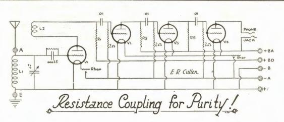
This week's receiver is one of intense interest to everyone at the moment. As is stated, purity is the keynote. Again it is inexpensive to build costing much less than the standard transformer coupled receiver. Our circuit to-day is a detector and three stages of audio frequency amplification. One condenser suffices for tuning, thereby ensuring simplicity of handling.
