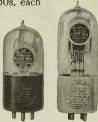
D.V.3 Filament, 3 volts .06 amp. Both Types Fit Standard American Socket. D.V.2 Filament 5 volts 25 amp.
