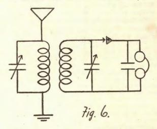
about a 75 turn for 2FC. In this circuit there are no losses due to end turns owing to the large coil not being in electrical connection to the small one when not in use. The variable condenser tunes the coils irrespective of which are in use, thereby providing the finest tuning. It must not be as-
