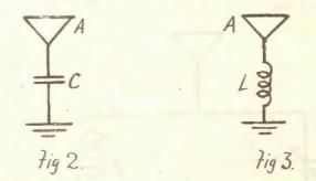
when used as a receiver, when the capacity and inductance bear a certain relation to one another, or are balanced. In this condition we are getting maximum current into the receiver and this is the aim of our receiver design. It follows then that a circuit containing definite capacity is better as in Fig. 4. This circuit has many advantages, besides the points already mentioned.
