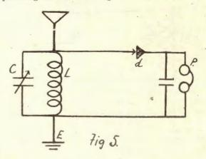
sumed that this circuit arrangement will give any greater selectivity, for this cannot be obtained with single coil tuners, owing to the fact as before mentioned, of the circuit being so tightly coupled. This is the reason why so many have found that one of
