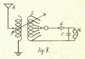
as far as operation is concerned. The first thing noticed is that it contains one of the faults of a single coil tuner, that is, end turn losses, and also as it has to be put into certain positions, it has to be wound with fairly fine wire, hereby increasing the damping or making it more broadly tuned.
