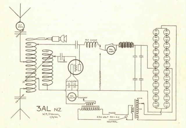
Diagram of Circuit used at Z3AL.
