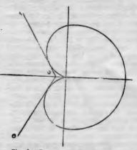
Fig. 2. Directional Characteristics of Single Loop
