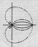
Fig. 3. Directional Characteristics of One, Two and Three Loops
