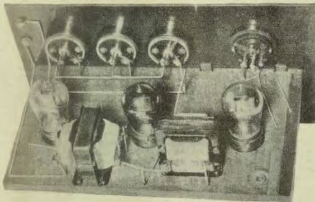
The Layout for the Audio-Frequency Part of the Inverse Duplex.
