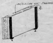
Fig. 10 - Finished condenser.
