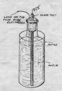
Fig. 8,-The completed resistance.
