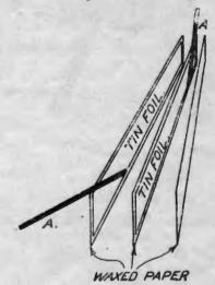
cut the tinfoil into two long strips the size required, and rolling them up together using as the dielectric good quality paper previously soaked in paraffin wax. The strips of paper should be  $\frac{1}{2}$  inch larger all round than the sheets of foil. Be-
