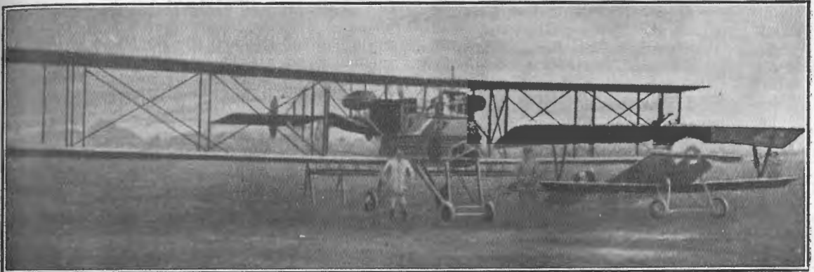
ONE OF THE FAMOUS FRENCH BREGUET BOMBING MACHINES, WITH A "NIEUPORT CHASER," WHICH, HAVING FAR GREATER SPEED THAN THE HEAVIER MACHINE, ACTS AS ITS GUARDIAN WHEN ALOFT.
