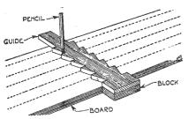
A Marker for Laying Out Divisions on a Board Lengthwise
