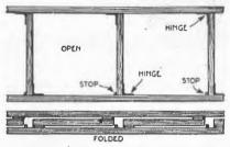
A Ladder with Folding Steps So That It Can Be . Stored in a Small Place
