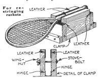
The wooden vise jaws are hinged to the bench and drawn together with a stovebolt and wingnut. Leather facings are glued on to protect the racquet handle from injury.
