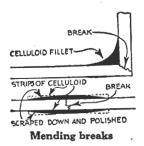
First cement the parts together in the ordinary way, so that they will hold temporarily. Then, with the celluloid mixture work a fillet or filling into the angle to act as a reinforcement, putting the putty on over a coating of cement. Although this dries rather slowly, it gets hard and makes a good job.
