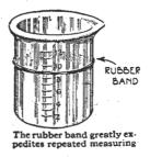
By placing a rubber band at the level wanted, it is possible to quickly pour the liquid to that point, as rubber is easier to see than the graduations would be.
