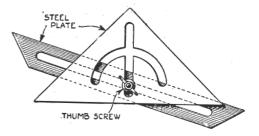
A Bevel Gage for the Mechanic Which Can Be Used for All-Around Work
