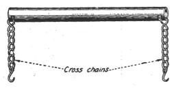
Pipe and Two Chains Make a Convenient Handle for Carrying a Storage Battery
