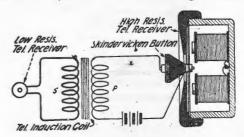
the receiver to a wooden base. Now make a brass bracket of the form shown, drill and tap a hole at the place indicated. Remove a carbon from an old flashlight battery and solder it by its brass cap to the end of a piece of threaded rod. Run the rod through the hole in the bracket and put a hard rubber knob on the other end. Make connections, as shown, to a battery, telephone induction coil and low resistance telephone receiver, and the amplifier is ready to amplify.
