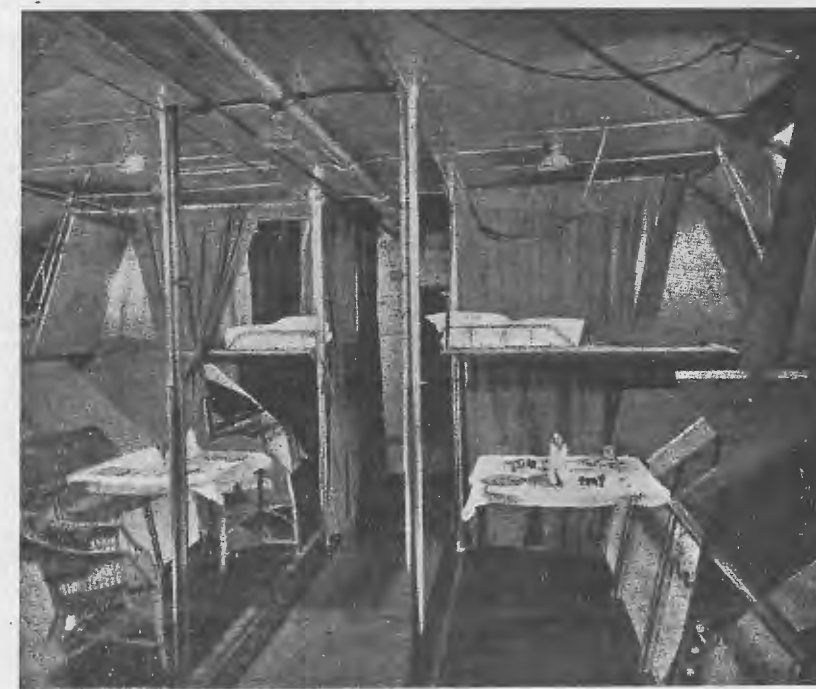
"R.36": Interior of the passenger car, showing the method of suspending beds and of unfolding mirror so as to make a table for the daytime. Bed folded away is seen on the extreme left of picture.
