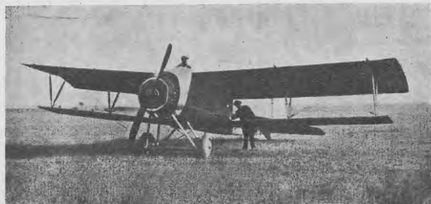
Front View of the Experimental Machine of Messrs. Gastambide and Levavasseur. The Wings are fully open.
