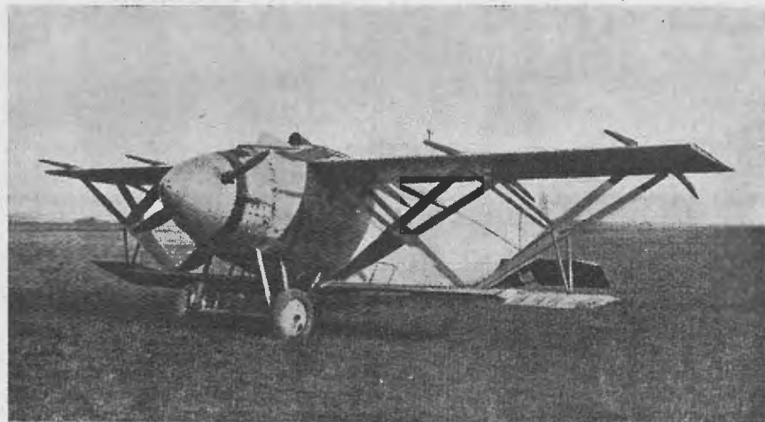
The Commercial Gastambide-Levavasseur Machine, showing the wings closed.
