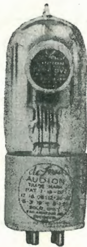
D.V. 2 Filament, 5 Volts, 25 Amp.
