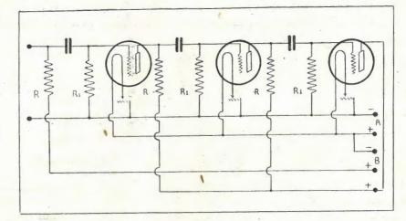
High plate voltages should be used with this form of coupling as part of the plate battery energy is dissipated by the high resistance in series with the battery and the plate of the tube. For the usual detector using 22½ volt it will be found desirable to use about 45.
