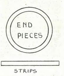
of two hard rubber rings with eight hard rubber strips connected to them, as shown in the drawings. Bare wire may be used, and in fact is preferable to insulated wire, as there is distributed capacity between turns. Number 18 or 20 copper wire may be used and should be annealed so as to be handled very easily.
