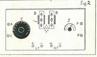
Index to Figures 1, 2 and 3. A: Aerial. B: Grid Coil. C. Twenty-three Plate Variable Condenser. D: Reaction Coil. E: Earth. F: Grid Condenser. G: Grid Leak. H: Valve. I: Valve Holder. J: Filament Rheostat. K: Low Tension (A) Battery. L: Fixed Condenser across 'phones. M: High Tension (B) Battery. P: Telephone Receivers. Figure 1: Schematic Diagram of connections.
