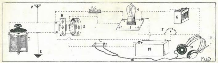
Figure 3: Illustrates the various component parts of receiver and how same are connected. The dotted lines indicate connecting wires.
