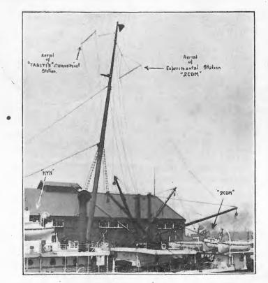
The above is a photograph of the after portion of the "Tahiti," in which may be seen the experimental wireless cabin (2CDM), its aerial and portion of that of the commercial station (MYN).
