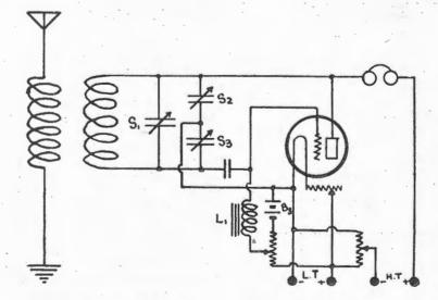
Diagram of the receiving circuit used by Mr. Slade.
