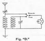
shown in Figure D. The only extra piece of apparatus is a single slide switch, which is almost certain to be found amongst the varied pile of junk which collects around every live experimental statich. Leave the switch so that the detector and telephones are connected to the aerial circuit, and when a station is tuned in switch over to the coupled connection and adjust the secondary resonance. With slight modification this circuit may be adapted for use with a valve receiver.
